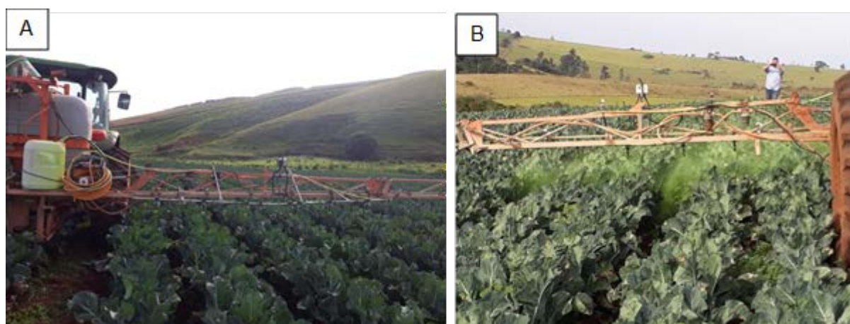
Figure 1. Electrostatic spraying system (A) and traditional spraying system (B)
