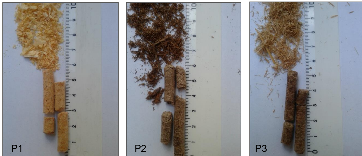
Figure 1. Pellets produced from biomass: P1: pine; P2: sugarcane bagasse; P3: bamboo
