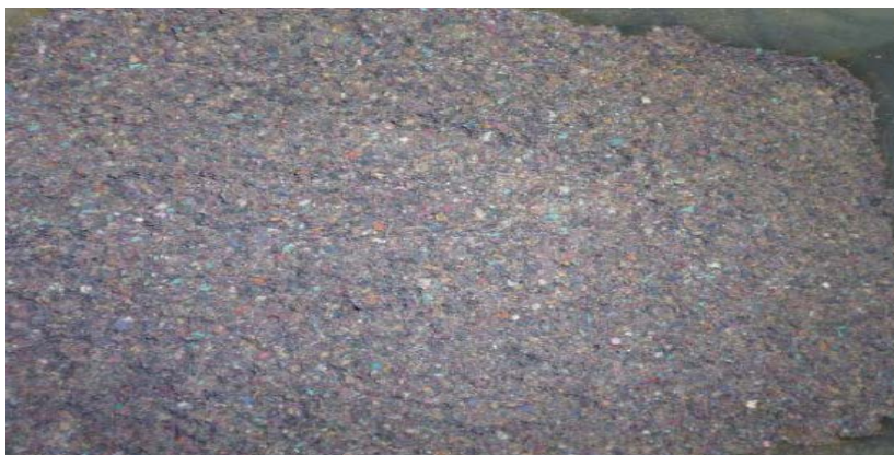
Figure 1. LSW samples after grinding and sieves
