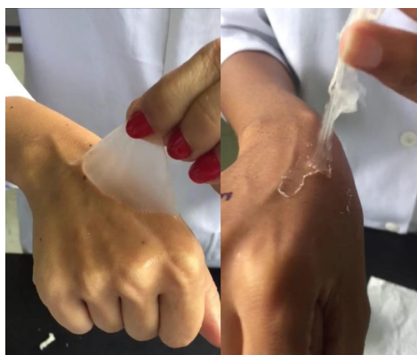
Figure 1. Removal of the film formed after drying. (A) Complete removal of formulation 4 film applied to the back of the hand without leaving residue. (B) Formulation 3 with a brittle, thick film and sticky consistency. Source: author's own work.
